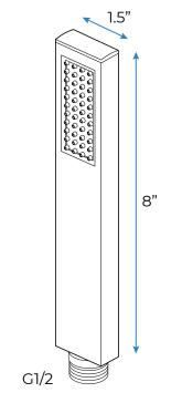
Flow Rate: 2.0 GPM / 7.6 LPM
